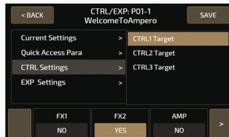
The 9 Ampero Mini effects modules are listed in the panel. with yes and no below each module to show if the CTRL 1-3 are activated or not. In the example image above, FX2 is controlled by the CTRL 1. Press to change between yes/no, and press the arrows on the right/left to scroll through the modules.
