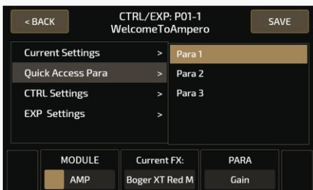
Use MODULE to select the target module. If you don't want the quick access para on, select OFF to turn its function off.
